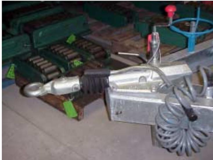
The British eyeshafts have a round or toroidal section eye and are used with a parallel type pin with sufficient clearance in the eye to permit the correct sequence of towing on the pin and braking on the jaw. If the pin is too large or the clearance between the jaw and pin too great, then both towing and braking loads will be put onto the pin.
